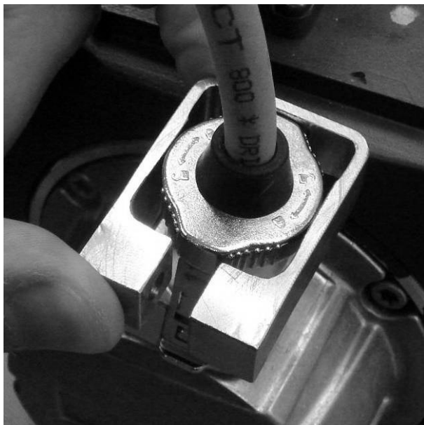
Fig. 2: Next, the disconnection protection device must be slid over the locking device.
