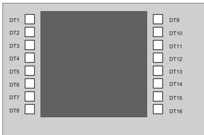
Figure 5-1 Assignment of the direct keys to the vertical softkeys of an operator panel front
