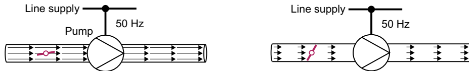
Figure 8-82 Flow control with pump and throttle connected to a 50 Hz line supply
