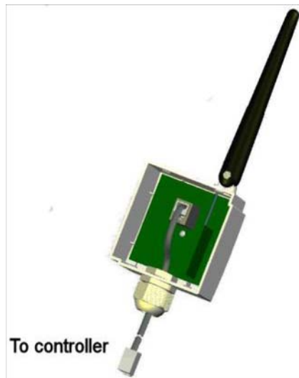
Figure 27: Telephone Socket Location
