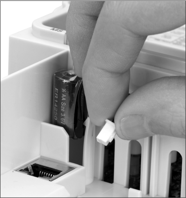
Figure 1. RTC battery connection
