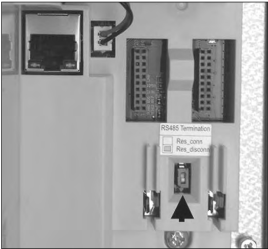
Figure 8. Termination resistor and shielding
