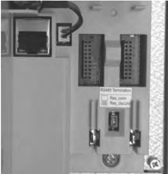
Figure 21. RS-485 Bus termination setup
